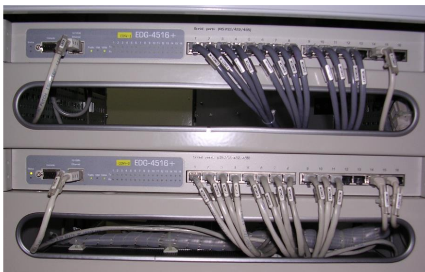
Figura 13 - Conversor EDG-4516+, RS232 / Ethernet.
